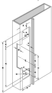
**7119, 7319** Hollow Metal & Wood Frames, 1-1/2" D **4119, 4319** Hollow Metal & Wood Frames, 1-1/2" D Not available in modular program
