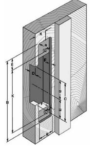
**7107**, **7307** Aluminum & Wood Frames, 1-1/2" D **4107**, **4307** Aluminum Frames, 1-1/2" D Any modular **A41**, **A43**, **A71** or **A73** with **B4707** faceplate
