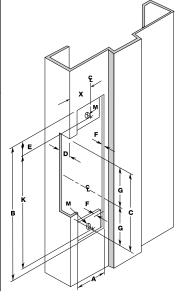
**7108, 7308** Aluminum & Wood Frames, 1-1/2" D **4108, 4308** Aluminum & Wood Frames, 1-1/2" D Any modular **A41, A43, A71** or **A73** with **B4708** faceplate
